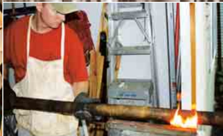
Bamboo culms are heated (above), split with a mallet and butcher's knife (facing page), and then carefully milled to precisely 60 degrees (top).
